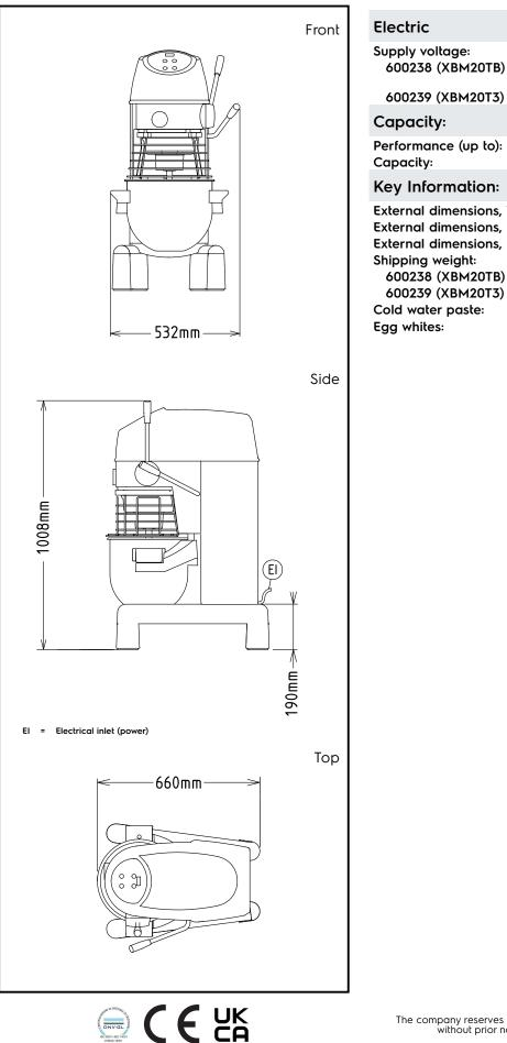
200-240/380-415 V/3 ph/50 600239 (XBM20T3) Ηz 6 kg/Cycle 20 litres External dimensions, Width: 521 mm External dimensions, Depth: 685 mm External dimensions, Height: 1010 mm 600238 (XBM20TB) 95 kg 600239 (XBM20T3) 94 kg 6 kg with Spiral hook
